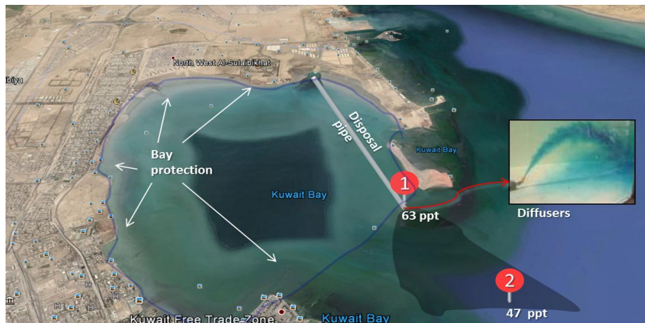
Figure 4. Suggested solution for brine disposal method for Kuwait bay
