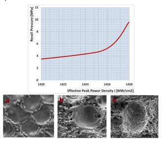
Figure 2: Recoil pressure variation with effective peak power density [16].
