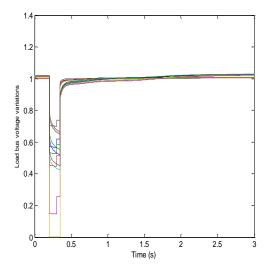
Figure 12: Variations of bus voltage with multiple STATCOM.
