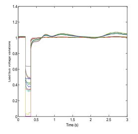
Figure 8: Variations of bus voltage with single STATCOM.
