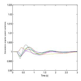
Figure 11: Variations of angular speed with multiple STATCOM.
