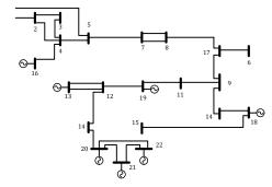
Figure 2: 7 machine 22 bus system.
