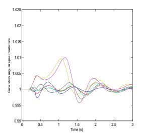
Figure 9: Variations of angular speed with multiple SSSC.
