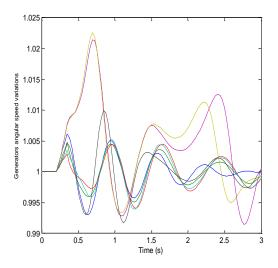
Figure 7: Variations of angular speed with single STATCOM.
