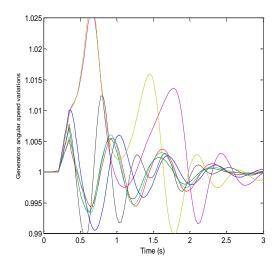
Figure 5: Variations of angular speed with single SSSC.
