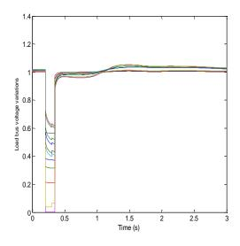
Figure 10: Variations of bus voltage with multiple SSSC.
