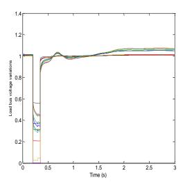
Figure 6: Variations of bus voltage with single SSSC.
