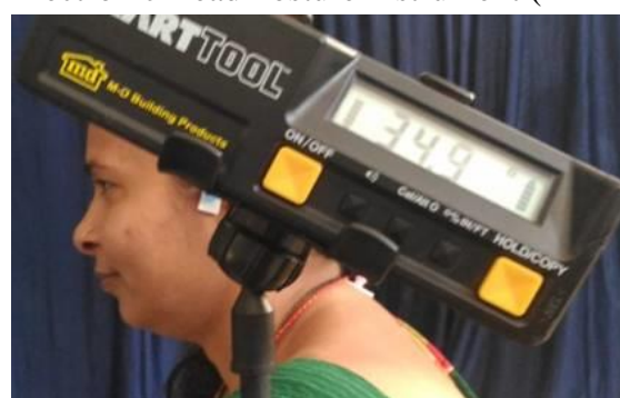
Figure - 3: Measurement of CV angle using Electronic Head Posture Instrument (EHPI).
