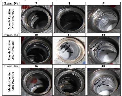
Figure 6: Moulds cavities after thermal friction drilling operations
