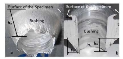
Figure 2: a) Bushing height (ha) and b) bushing wall thickness (tw), on the bushing shape
