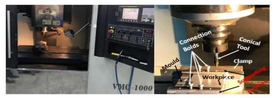
Figure 1: a) CNC milling machine and its computer screen, b) experimental setup
