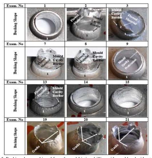
Figure 5: Bushing shapes achieved from thermal friction drilling with mould and without mould
