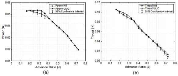
Figure 2: Power-(a) and thrus-(b) vs advance ratio experiment data from KIT and UIUC including 95% confidence interval
