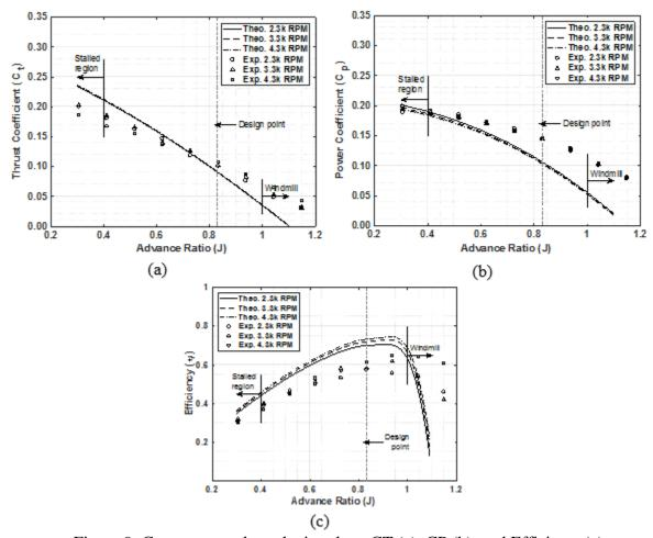
Figure 9: Constant angular velocity plots: CT (a), CP (b), and Efficiency(c)
