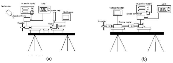
Figure 1: Experiment set up for Thrust (a) and Torque (b)
