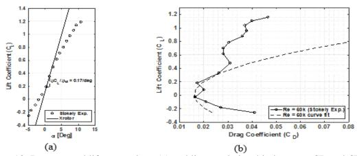
Figure 13: Recomputed lift curve slope (a) and linear relationship between CL and CD (b)
