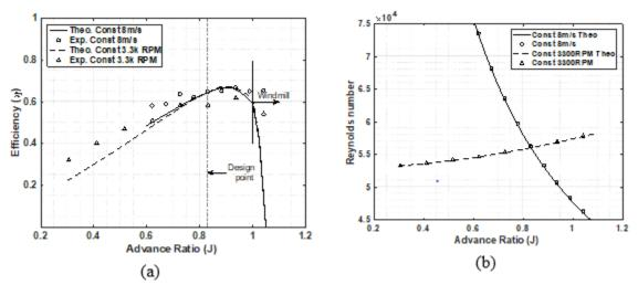
Figure 15:  $\eta$  vs J (a) and Reynolds number vs J (b) for  $\delta$ CL/ $\delta\alpha$  = 0.17
