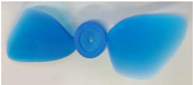
Figure 6: 3D printed propeller
