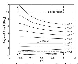
Figure 8: AoA vs station radius at constant angular velocity of 3300RPM.
