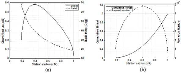
Figure 5: Iterated propeller geometry (a) and Re distribution (b)
