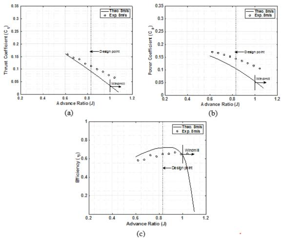
Figure 10: Constant 8m/s constant Velocity plots: CT (a), CP (b), and Efficiency(c)
