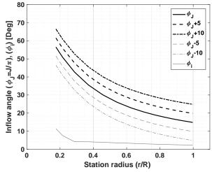
Figure 11: Inflow angle  $(\phi J=J/\pi)$  Vs blade station radius r/R
