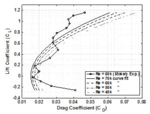
Figure 4: CL vs CD relationship with changing Reynolds number for SD7037.
