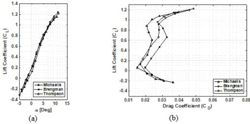
Figure 16: CL Vs α (a) and CL Vs CD (b) for SD7037 at Re=60k
