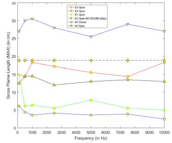
Figure 11: Varying Maximum Gross Flame Length with frequency
