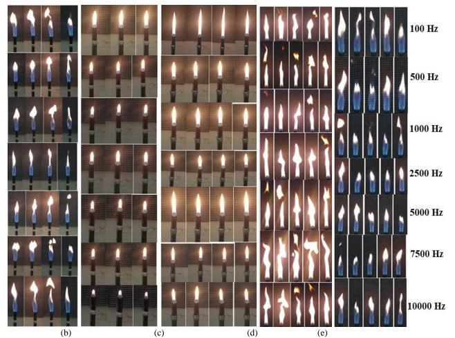
Figure 9: Variation in flames with varying sound wave's frequencies for varying air entrainment configurations
