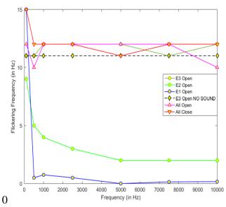
Figure 12: Variation of Flame Flickering frequency with Acoustic frequency
