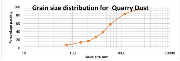
Figure 2: Percentage passing against sieve sizes (quarry dust)
