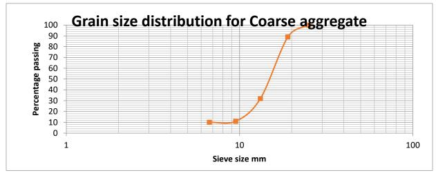
Figure 3: Percentage passing against sieve sizes (Coarse aggregate)
