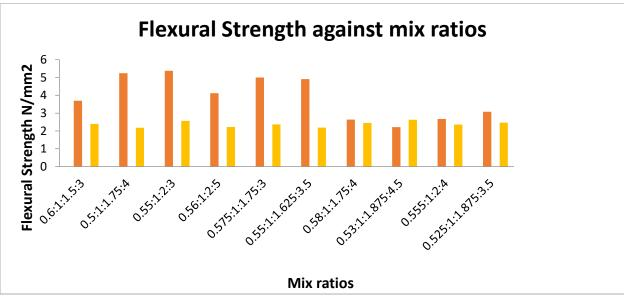
Figure 3: flexural strengths against mix ratios
