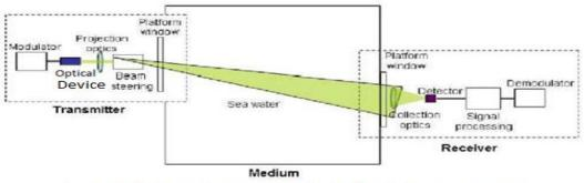
Figure 2 : Block Diagram of a Underwater Optical Communication System(UWOC)
