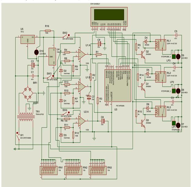
Figure 3: overall circuit design of the petroleum monitoring system
