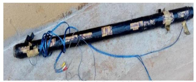
Figure 1: Sample petroleum pipeline coated with sensor wires
