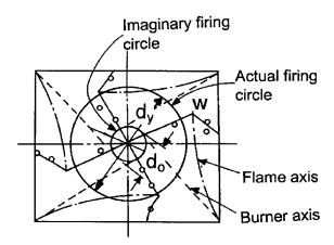
Figure 3: Tangential Velocity Distribution in a Tangential Boiler
