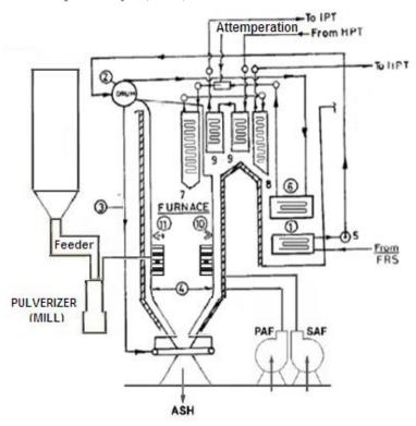
Figure 1: Layout of Tangentially Fired Boiler
