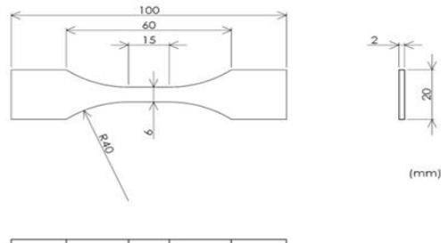
Figure 4: Specimen for a tension test which was cut down from the CFRP circular
