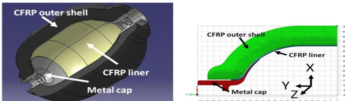
Figure 7: Finite-element-method analysis model of CFRP container fabricated by FW method
