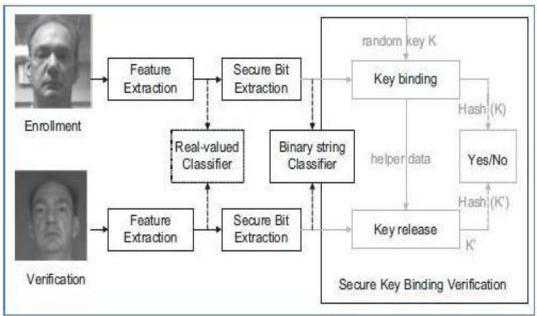
Figure 2: Overview of template protected biometric verification system [4]
