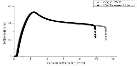
Figure 1: Original and blend tensile stress-strain curves
