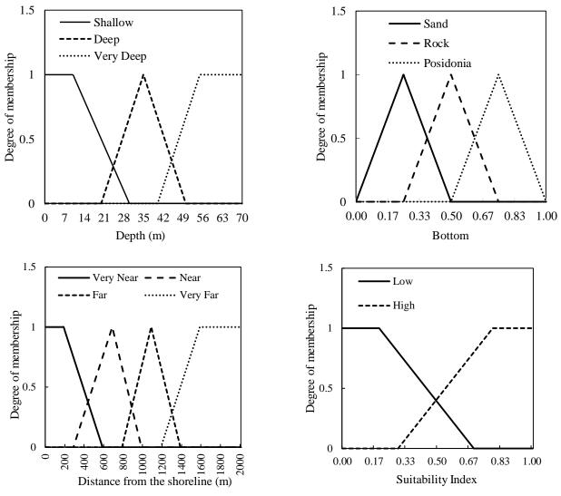
Figure 4: Fuzzification of input and output variables for the first stage.
