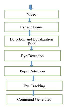
Figure 2: Image processing module
