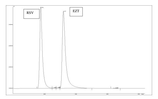
Fig 2: Chromatogram of mixed standard solution of RSV (10  $\mu$ g mL<sup>-1</sup>, RT = 1.71 min) and EZT (10  $\mu$ g mL<sup>-1</sup>, RT = 3.25 min)
