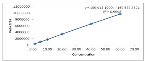
Fig 6: Calibration curve of Paracetamol
