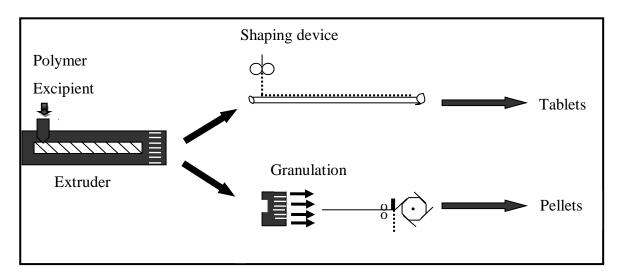
Figure 1.5: Scheme of hot melt extruder (Leuner and Dressman, 2000)
