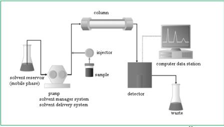
Fig.1.1: Components of HPLC instrument block diagram.<sup>22</sup>
