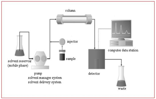
Fig.1: Components of HPLC instrument block diagram.
