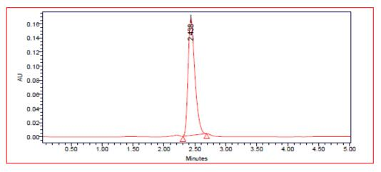
Fig. 3 Typical chromatogram of mixture of Standard solution
