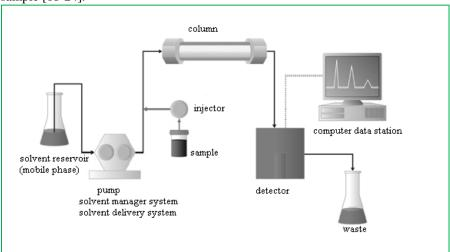
Fig.1: Components of HPLC instrument block diagram. <sup>22</sup>
