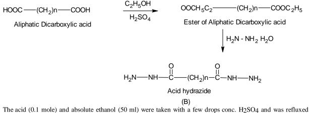
The acid (0.1 mole) and absolute ethanol (50 ml) were taken with a few drops conc. H<sub>2</sub>SO<sub>4</sub> and was refluxed for 6 hours. The reaction mixture was concentrated by distilling off the excess of ethanol under reduced pressure. The ester obtained was used for the preparation of hydrazide directly.
