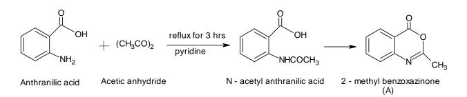
A Mixture of anthranilic acid (0.12 mol) in acetic anhydride (0.2 mol) with few drops of pyridine was refluxed for 3hr. The reaction mixture was filtered, washed and recrystallised from absolute ethanol, to get the crystals of 2-methyl 1,3,4- benzoxazinone(A). The physical data of compound (A) are summarized in **Table-1**.
