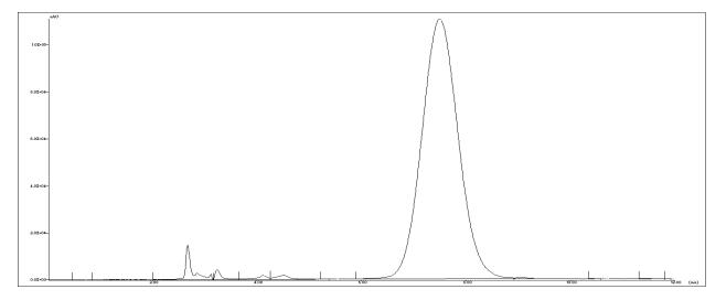
Fig. 7: Representative Chromatogram of Photolytic Degradation (20 µg/ml)
