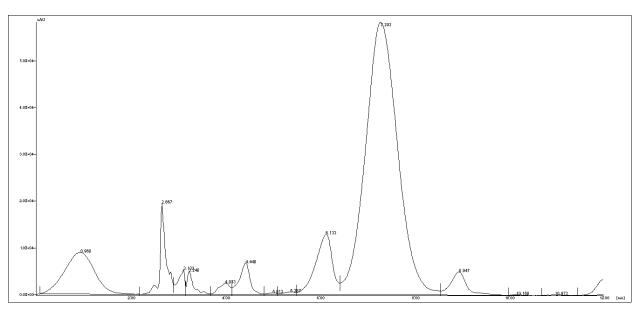
Fig. 4: Representative Chromatogram of Alkaline Degradation (20 µg/ml)
