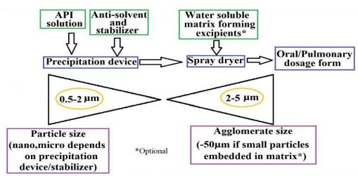
Fig. 1: Schematic representation of manufacturing flow for a bottom-up process
