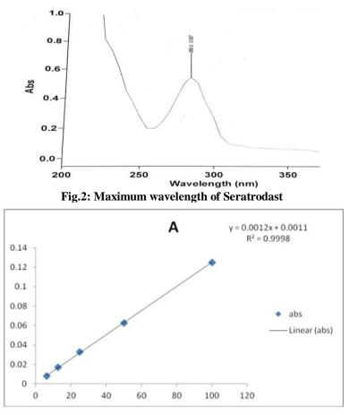
Fig.3: Calibration curve of Seratrodast
