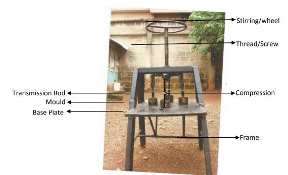
Plate 1.0: The fabricated screw press.
