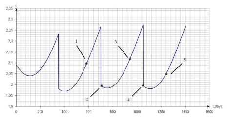
Fig. 1 - Dependence the objective function *J* optimal values on the NPP operation time with full burning-up of nuclear fuel **Conclusions**
