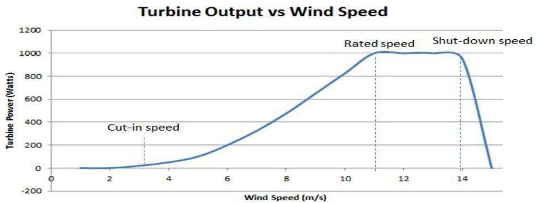
Fig. 8 Performance curve of Darrieus wind turbine [13]
