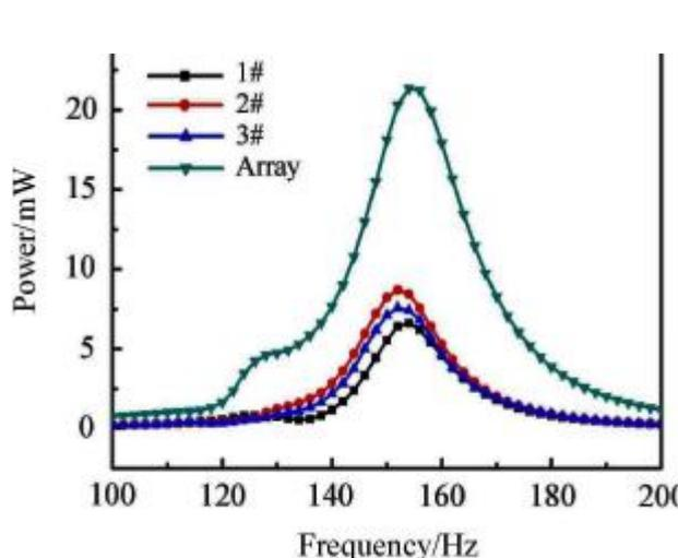
Fig. 12 Generated power using circular diaphragm array in parallel connection [24]
