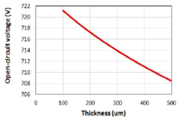
Fig. 5 Open circuit voltage vs thickness
