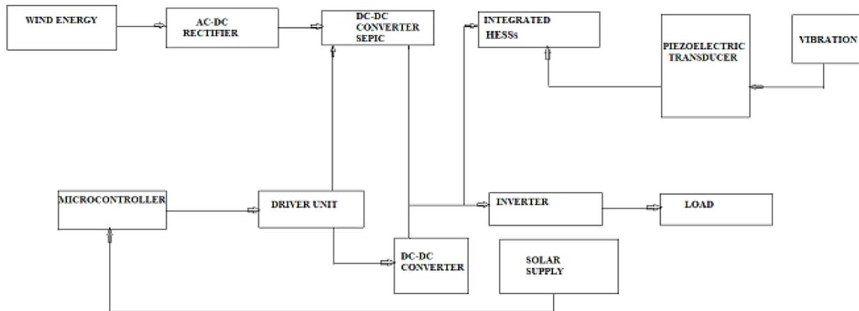
Fig. 15 Block diagram of the Proposed Model of the Integrated System for Energy Harvesting
