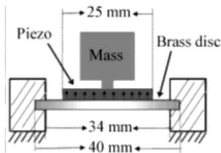
Fig. 10 The detail of single circular piezoelectric diaphragm array structure
