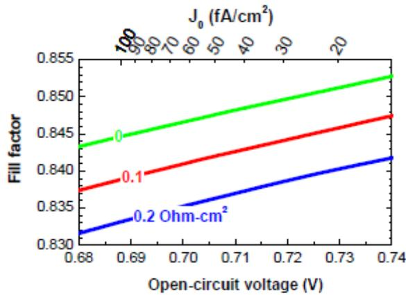
Fig. 2 Fill factor open circuit voltage [5]
