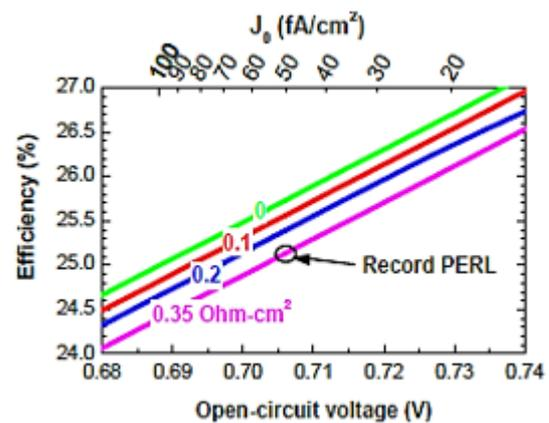
Fig. 3 Efficiency vs open circuit voltage [5]
