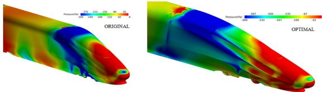
Fig. 9 Pressure distribution near head-coach for optimal and original design [14]
