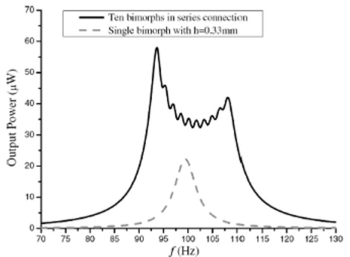
Fig. 13 Generated power level using multiple bimorphs [22]
