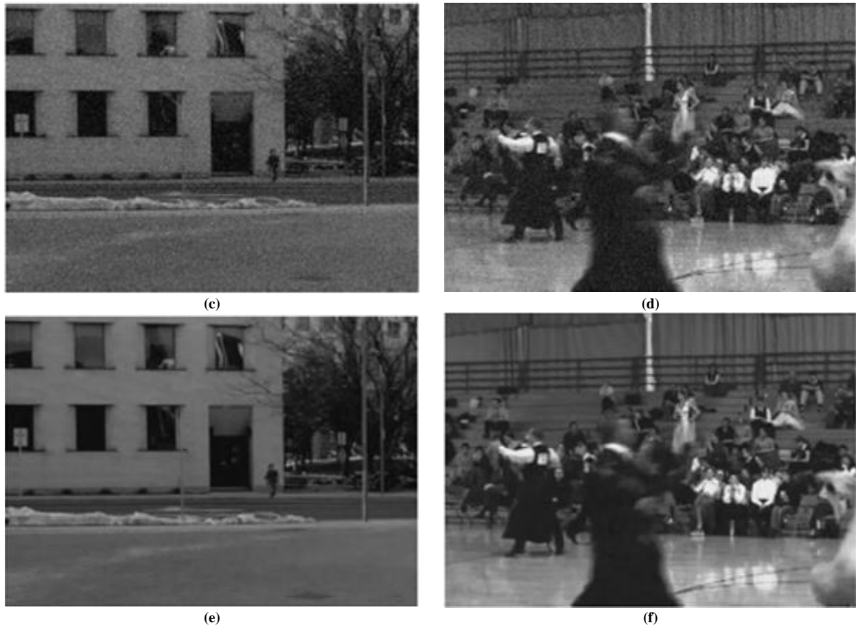
Fig. 3 Examples of VBM3D filtering: The two test videos vassar and ballroom are already being degraded by Gaussian noise signal with \sigma = 20 , and (a),(c),(e) in that order are original, noisy and the denoised frame for vassar and (b),(d),(f), respectively are original, noisy and the denoised frames for the ballroom
