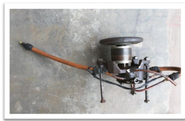
Fig. 12 Compressor running at 28 psi
