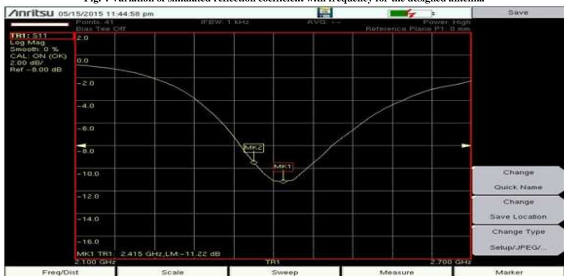
Fig. 5 Variation of measured reflection coefficient with frequency for the designed antenna
