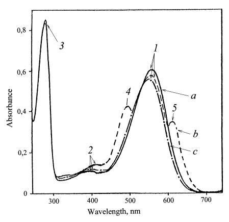
**Fig. 8.** The absorption spectra of the PM (50% (v/v) ethanol) at various stages of processing: (a) – natural BR; (b) – PM after intermediate treatment; (c) – PM purified from carotenoids. The bandwith (1) is the spectral form of BR $^{568}$ , (2) – impurity of spectral form of metabacteriorhodopsin (M $^{412}$ ), (3) – the total absorption bandwith of aromatic amino acids, (4) and (5) – extraneous carotenoids. As a control used the native BR
