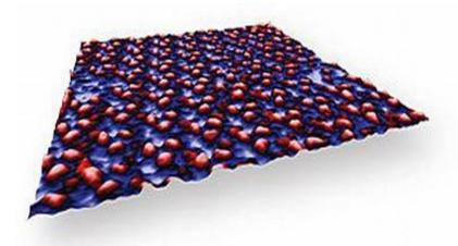
**Fig. 7.** An artificial membrane from the BR-containing PM in scanning electron microscope (SEM): scanning area  $-100 \times 100$  mm, resolution -50 nm, magnification -100000 times. PM shown in purple, BR - in red color
