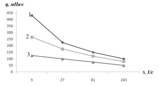
Figure 2: The Dependence of the Effective Viscosity of the VPN Speed Shift at Different Temperatures: 1 – 27 °C; 2 –30 °C; 3 – 35 °C
