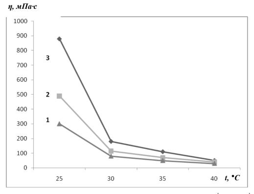
Figure.1: Zavisimost Effective Viscosity of the Vpntemperature at Shear Rates of: 1 27  $c^{-1}$ ; 2 – 81  $c^{-1}$ ; 3 - 243  $c^{-1}$
