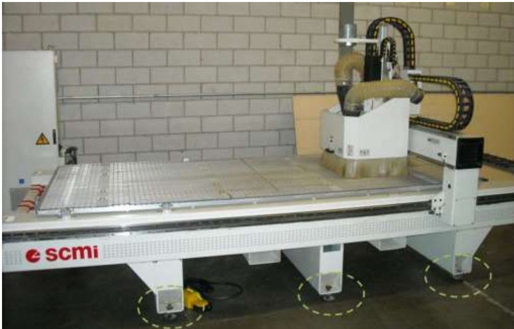
Figure 5. Machine tool with antivibration damper
