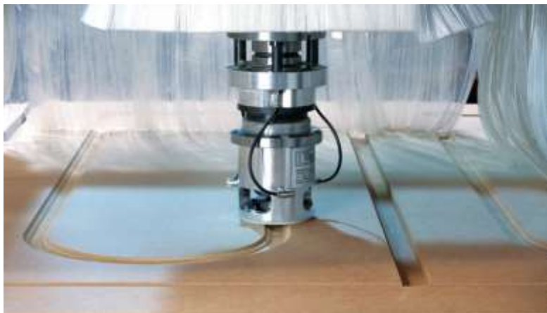
Figure 4. Use of flexible curtains in machine tools (Schmersal, 2016)
