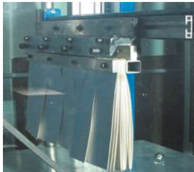
Figure 7. Barriers with 16-layers
