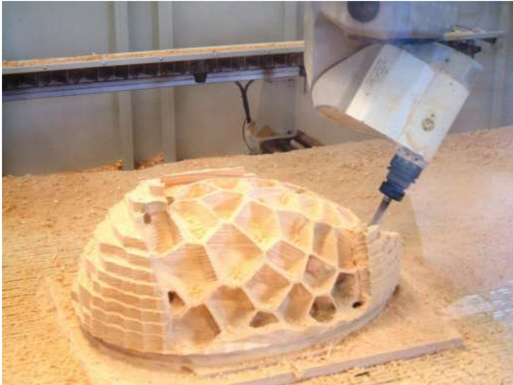
Figure 4. Production of complex geometry by woodworking [Courtesy SCM Group]
