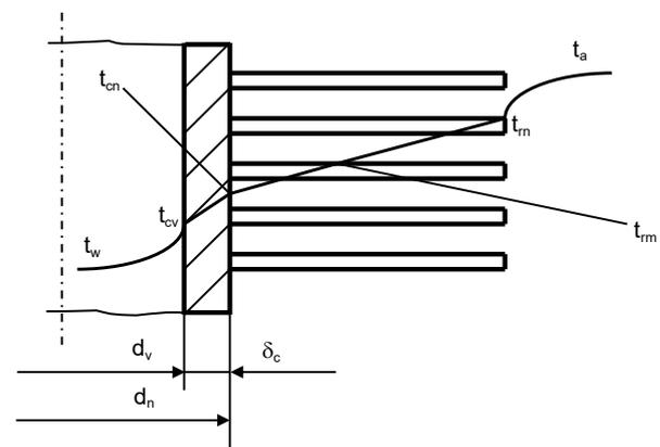
Fig. 1. Temperature variations on ribbed pipe
