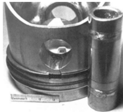
Fig. 5. Wear in the pin hole, [16]
