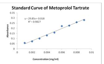
Fig. 1: Standard curve for metoprolol tartrate
