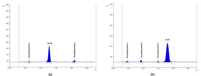
Fig. 2: Representative densitogram after acid treatment (a) TELMI with degradation products at Rf 0.13, 0.71 and (b) CILNI with degradation products at Rf 0.06, 0.26 and 0.47
