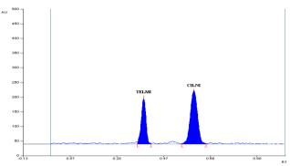
Fig. 1: Representative densitogram of mixed standard solution of TELMI (600 ng band-1,  $R_{\rm f}$  = 0.38  $\pm$  0.03) and CILNI (300 ng band-1,  $R_{\rm f}$  = 0.62  $\pm$  0.05)
