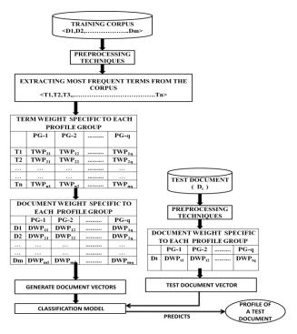
Figure.1 The architecture of PDW Model
