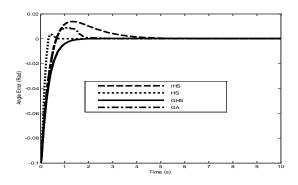
Figure 9. Angle errors for inverted pendulum (HS, GHS, IHS and GA)
