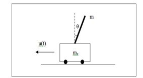
Figure 7. Inverted pendulum system
