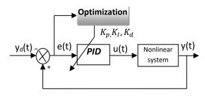
Figure 6. Tuning of PID controller using HS algorithms
