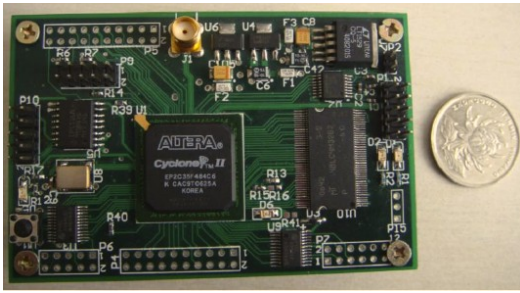
Figure 7 The circuit of FPGA Navigation computer ( 9 \times 6 \times 2\text{cm} )
