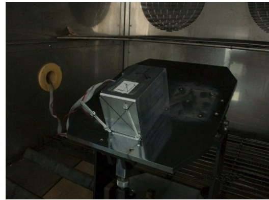
Figure 8 Thermal testing for MEMS IMU
