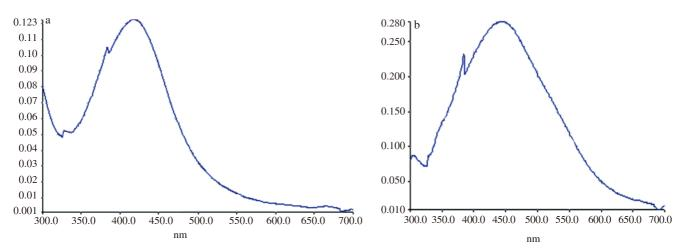
Figure 2. UV-vis spectra of silver nanoparticles synthesized from *A. indica* (a) and *E. scaber* (b) showing peak at near 420 nm because of surface plasmon resonance of silver nanoparticles.
