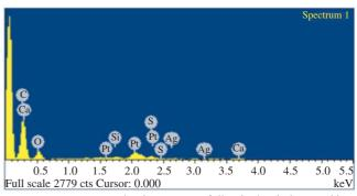
Figure 7. EDX spectrum showing presence of silver in chemical composition of larval body.
