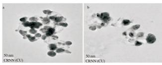
Figure 3. TEM images of quasi spherical silver nanoparticles synthesized from *A. indica* (a) and *E. scaber* (b).
