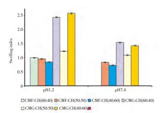
**Figure 3.** Swelling indices of the formulated CMF–CH or CMG:CH IPC films in pH 1.2 (2h)and pH 7.4 (24hrs). Data is represented as mean±SD.
