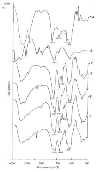
**Figure 1.** FTIR spectra of FG (A); CH (B); CMF (C); complex formed by interacting CMF and CH in the ratio of 60:40 (D); 50:50 (E) or 40:60 (F)
