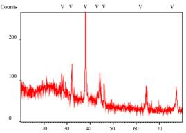
**Figrue 4.** X–ray diffraction analysis of biogenic silver nanoparticles from *A. bisporus*.
