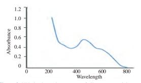
Figure 3. UV-vis absorption spectra of silver nanoparticles synthesized from V. serpens.
