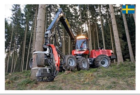
Figure 9. Forest harvesting with a modern, single grip, harvester with a capacity of up to 50 m<sup>3</sup> per machine hour.
