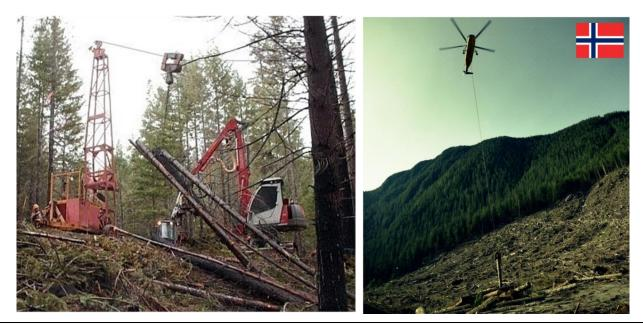
Figure 6. Logging by cable crane and transportation of logs from the site supported by helicopter.
