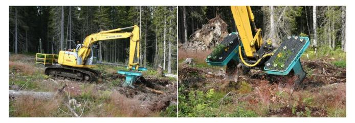
Figure 3. Self-propelled planting machines in Scandinavia can efficiently plant container seedlings on forest sites. The seedlings and machine were designed in concert, and in response to a dwindling, more expensive labor force. Photos by R. Kasten Dumroese
